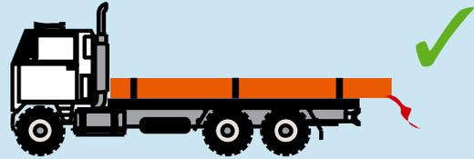
The overall length of a rigid truck must not exceed 12.5 metres (including any load). The overall length of a truck and trailer or prime mover and semi-trailer (including any load) must not exceed 19.0 metres.
