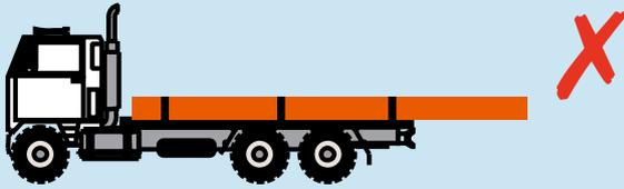
The maximum rear overhang of a rigid truck, including any load carried, is the lesser of 3.7 metres or 60% of the wheelbase, measured from the rear overhang line which is generally the centre line of the rear axle or axle group.
